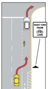
Buffer discontinued and bike lane line dashed 200ft before an intersection. Right-turning motorists must make turns from the bike lane and yield to bikes.
